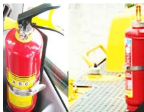
Manual Fire Extinguisher (Inside / Outside the Cab)
