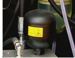
Accumulator for Boom lowering
