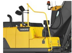
Access way with Handrail
