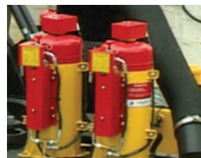
Automatic Fire Detection & Suppression System (AFDSS)
