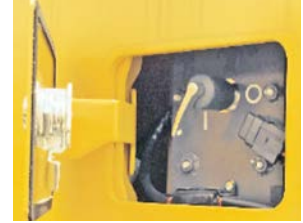
Battery cut-off switch
